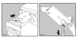
The reservoir must be re-inserted correctly.
